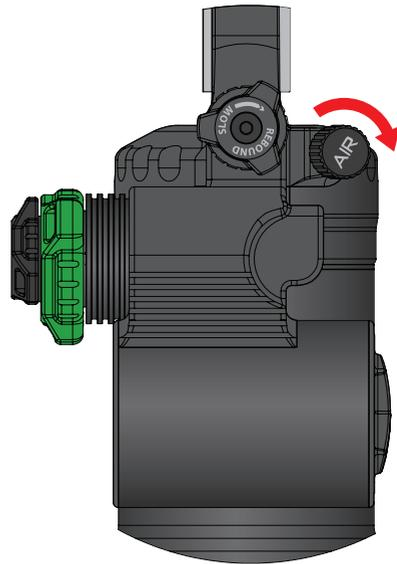
Note: Cycle the shock through its travel several times as you gradually increase pressure in the main chamber.
